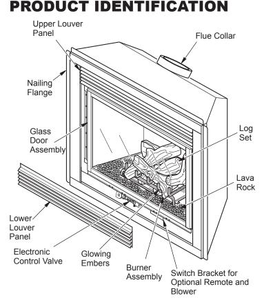
Figure 1 - Direct-Vent Fireplace with Electronic Ignition
